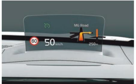
Makes driving safer by minimizing the movement of driver's line of sight
